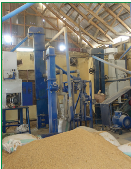
Large rice processor with an installed capacity of 15 M T per day.
