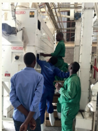
REACTS II team fixing the Grader and the De-stoner
