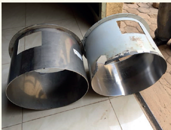
Worn-out Whitener Protection Ring that required replacement
